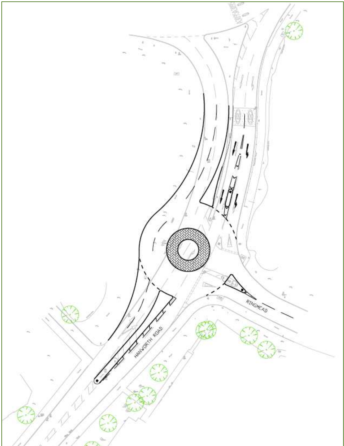
Figure 7: Hanworth Road / Ringmead Junction Improvement Scheme
